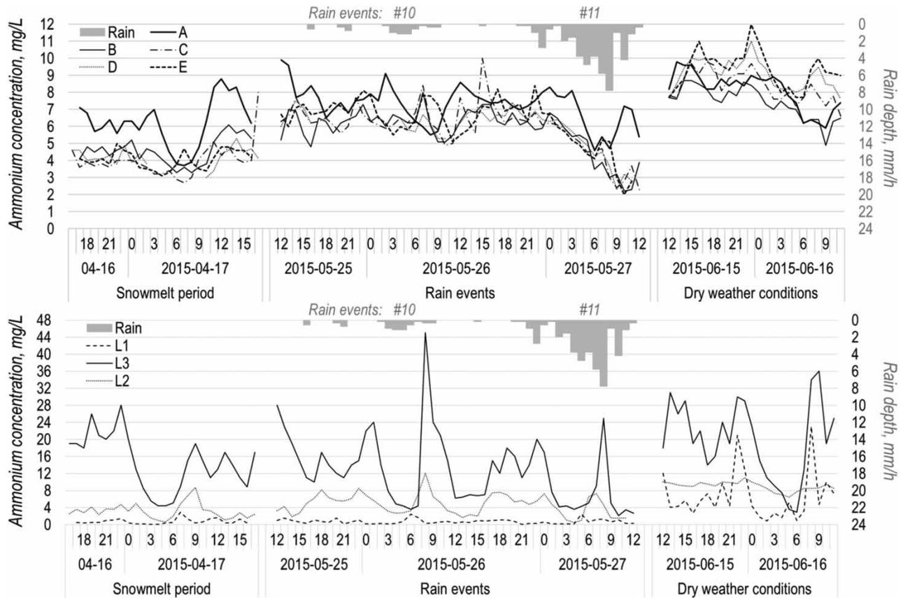
**Figure 3** | Ammonium concentrations sampled by automatic samplers (left axis) and rain depth (right axis) along the main sewer section (top) and in tributary sewers (bottom) during the snowmelt period (left-hand section), rain events #10 and #11 (centre section) and dry weather conditions (right-hand section).
