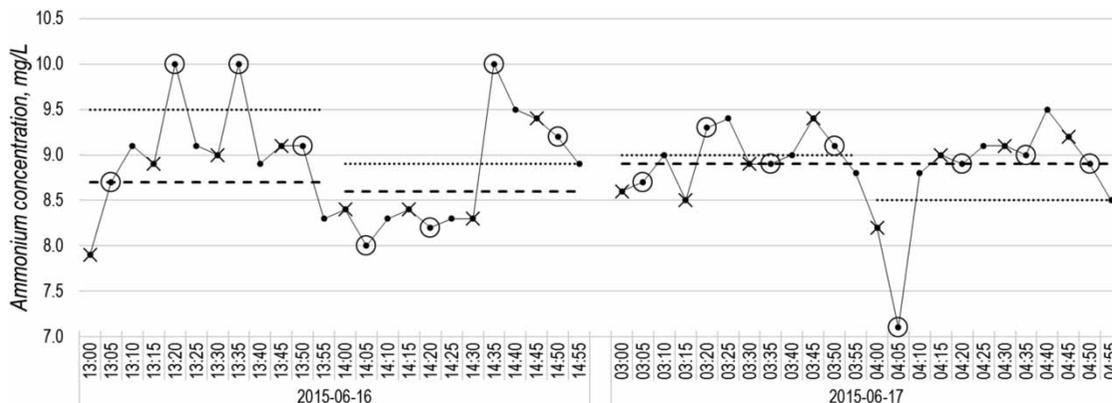
**Figure 5** | Ammonium concentrations in samples collected by the automatic sampler every 5 minutes during the daytime (left) and at night (right) at sampling station E. X- and O-markers indicate subsamples that would be taken during regular 15 min time-weighted sampling and same sampling with 5 min delay, respectively. Dashed and dotted lines show resulting average hourly sample concentrations for regular and delayed sampling, respectively.
