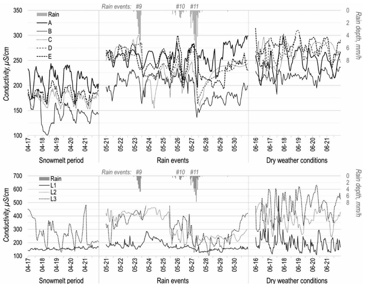
**Figure 4** | Conductivity measurements (left axis) and rain depth (right axis) along the main sewer section (top) and from tributary sewers (bottom) during the snowmelt period (left-hand section), rain events #9, #10 and #11 (centre section) and dry weather conditions (right-hand section). Note the difference in the left y-axis between top and bottom panels.
