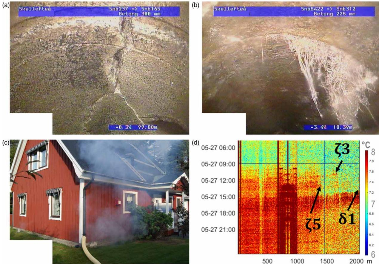
**Figure 2** | Examples of the results found from (a) CCTV – cracked pipe; (b) CCTV – roots penetration; (c) smoke inspection – roof misconnection (for location, see Figure 1(a),  $\epsilon 3$ ); (d) DTS – rain event #11 (for location, see Figure 1(a),  $\delta 1$ ,  $\zeta 3$ ,  $\zeta 5$ ).
