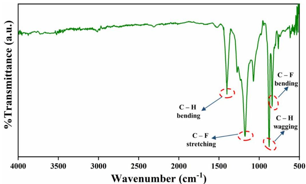
**Figure 3** | FT-IR spectra of the recycled PVDF beads.
