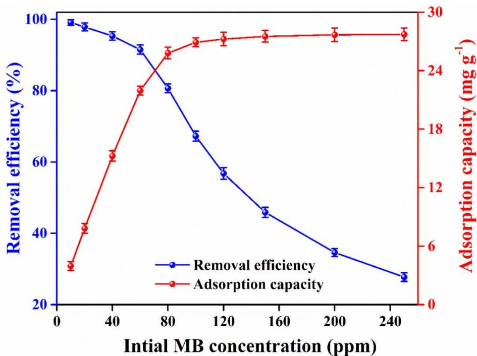
**Figure 7** | Removal efficiency and adsorption capacity of recycled PVDF beads with varying initial concentrations of MB dye (adsorbent dose:  $2.5 \text{ g L}^{-1}$ , contact time: 180 min, and pH: 7).
