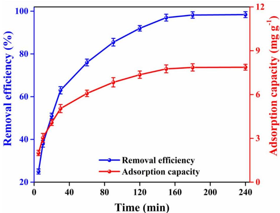
**Figure 6** | Removal efficiency and adsorption capacity of recycled PVDF beads with varying contact time (adsorbent dose:  $2.5 \text{ g L}^{-1}$ , initial MB dye concentration: 20 ppm, and pH: 7).
