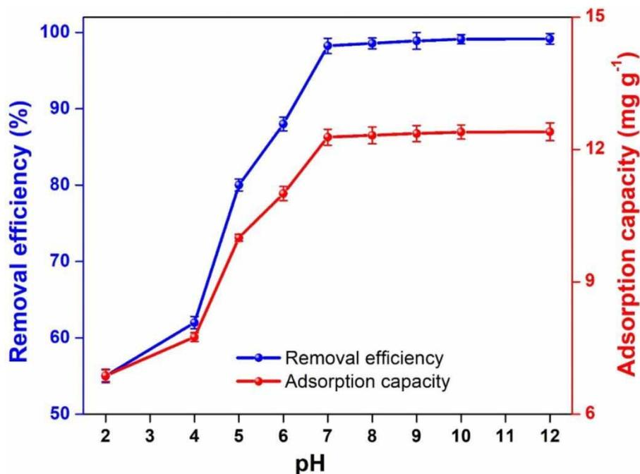
**Figure 5** | Removal efficiency and adsorption capacity of recycled PVDF beads with varying pH (adsorbent dose:  $2.5 \text{ g L}^{-1}$ , initial MB dye concentration: 20 ppm, and contact time: 180 min).
