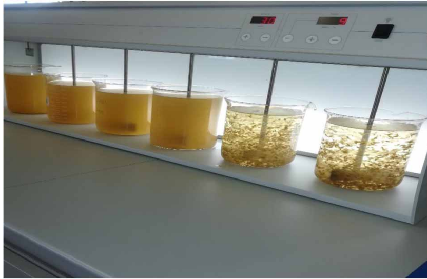
Figure 8 | Pictorial representation of floc formation during jar tests experiment.
