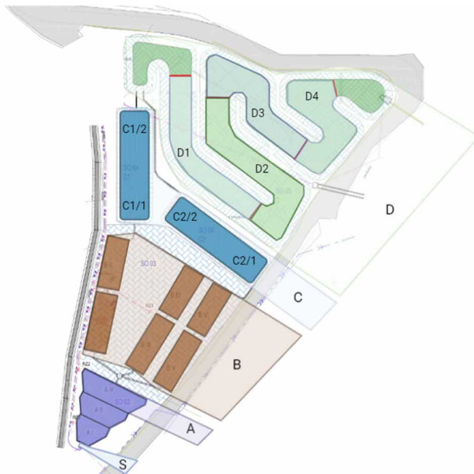
Figure 1 | Wetland+ modules. The inlet (S), aeration system including sedimentation (a), permeable reactive barrier remedial system (b), biosorption module (c), and aerobic wetland system (d).
