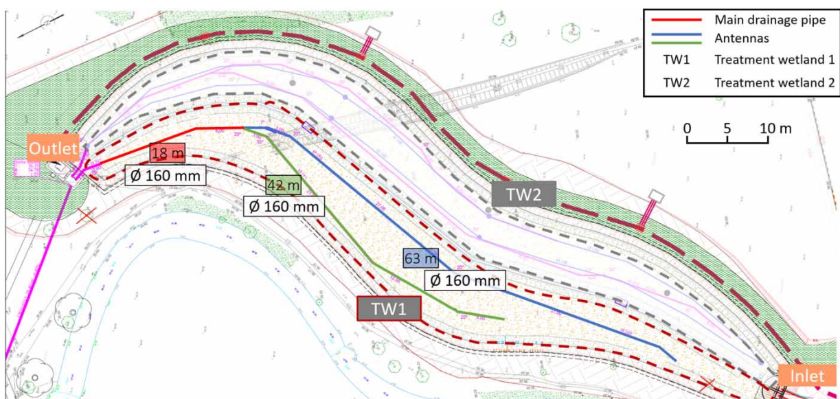
Figure 1 | Drainage system of the Life ADSORB TWs. The details of the underdrain network of TW1 are shown, while only the outline of the underdrain network of TW2 is shown in pink.
