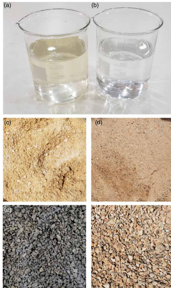
Figure 1 | Treated wastewater (a) and drinking water (b), natural sand (c), mixed recycled sand (d), natural gravel (e), and mixed recycled gravel (f) were used.
