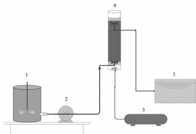
**Figure 1** | The general scheme of the pilot used in this research (1-Wastewater injection tank; 2- Injection pump; 3- Air compressor; 4- Bioreactor; 5- Secondary settling tank).
