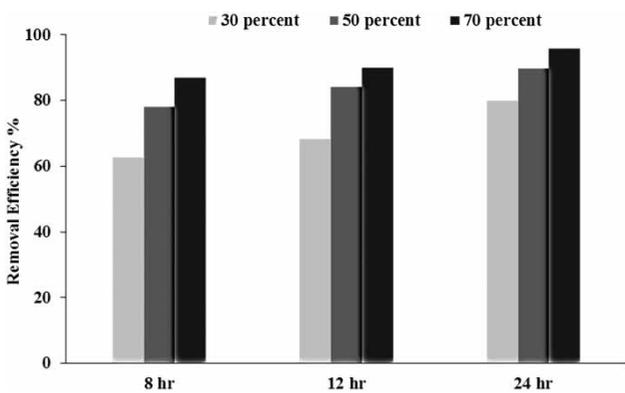
**Figure 3** | COD removal efficiency in 30, 50, and 70 percent reactor filling with  $k_1$  media (MLSS = 3,000 mg L<sup>-1</sup>).
