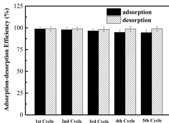
**Figure 8** | Adsorption and desorption efficiency of CF-SCB.
