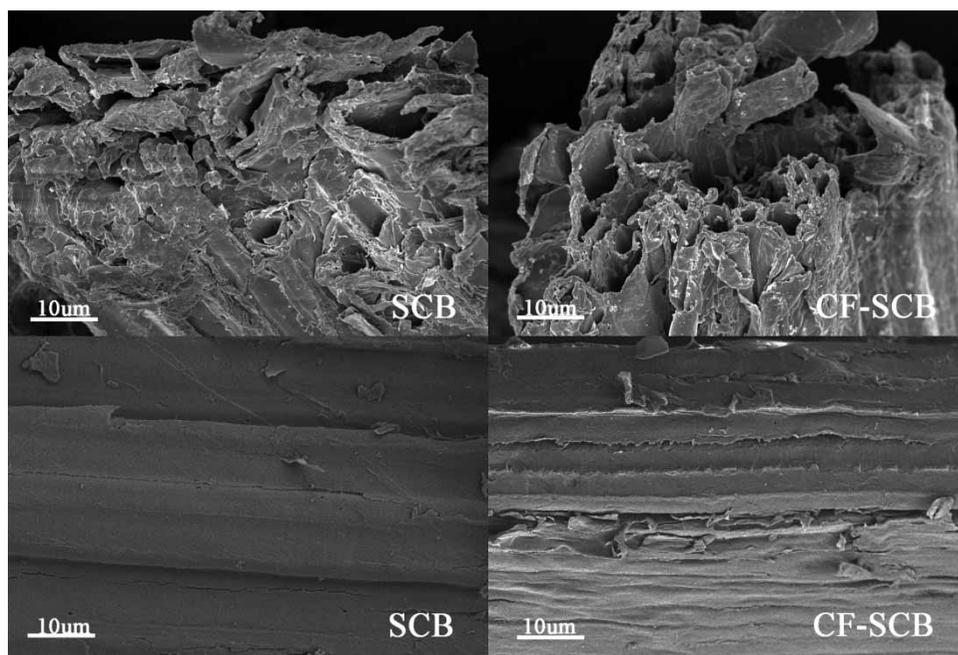
Figure 2 | SEM micrographs of SCB and CF-SCB.
