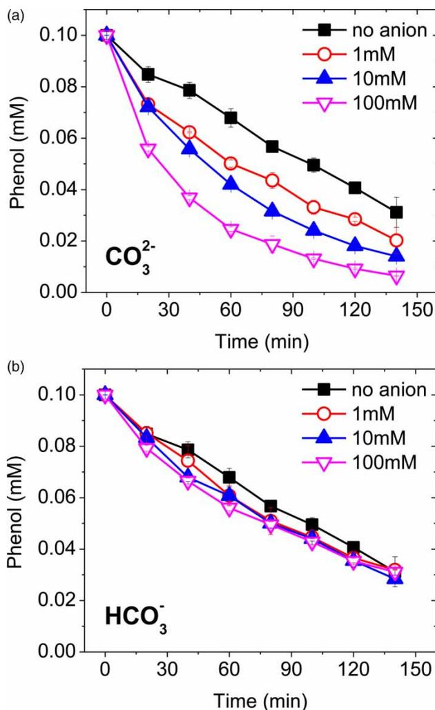
**Figure 4** | Impacts of  $\text{CO}_3^{2-}$  and  $\text{HCO}_3^-$  on phenol oxidation by TAP. Experimental conditions:  $[\text{PS}]_0 = 10 \text{ mM}$ ,  $[\text{Phenol}] = 0.1 \text{ mM}$ , and  $T = 50^\circ \text{C}$ .
