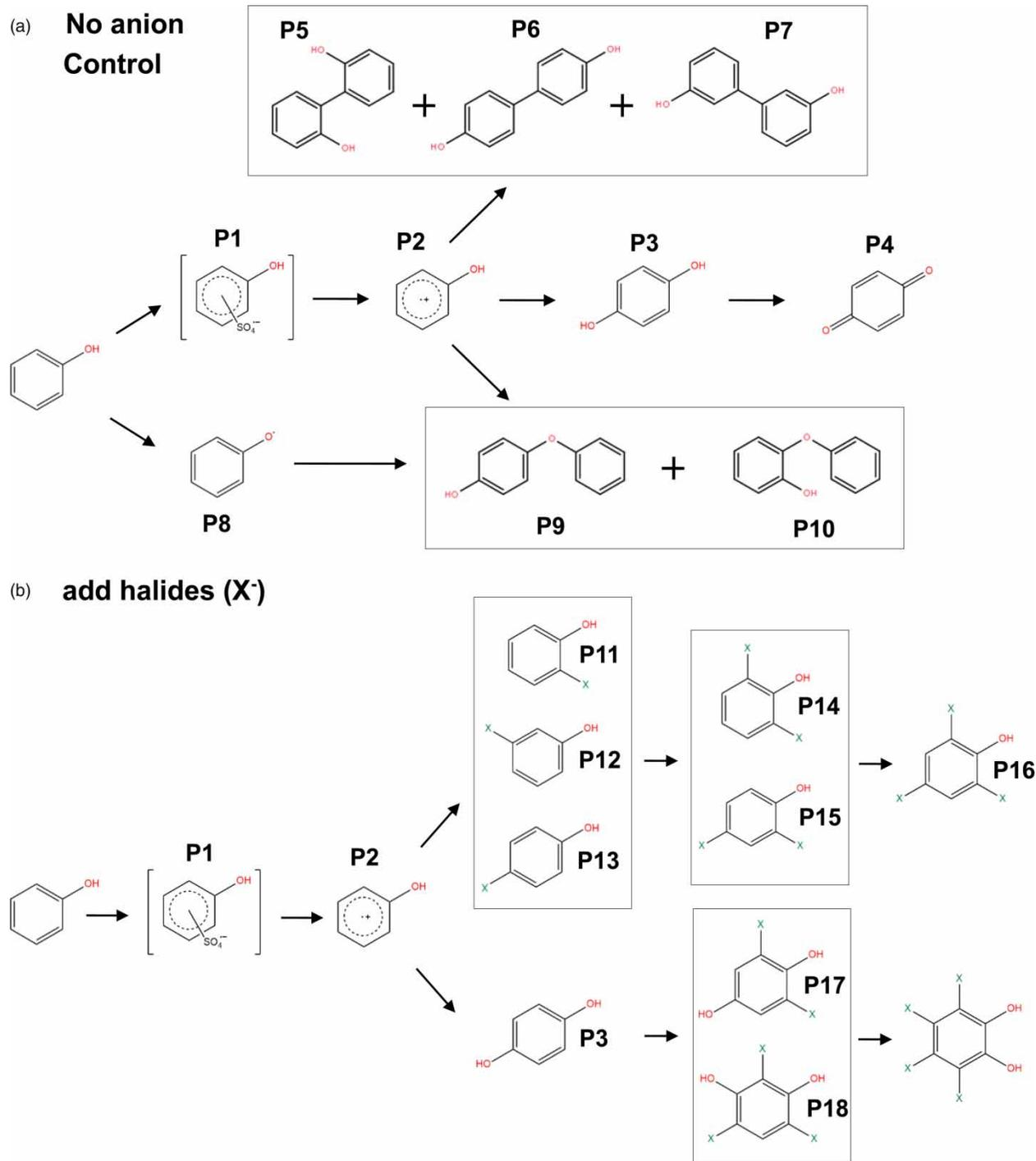
**Figure 6** | Reaction pathway in the control treatment without anions (a) and in the treatment containing halides (b).
