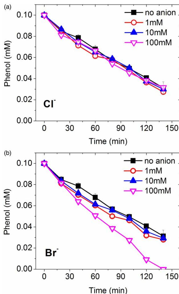
**Figure 1** | Impacts of  $\text{Cl}^-$  and  $\text{Br}^-$  on phenol oxidation by TAP. Experimental conditions:  $[\text{PS}]_0 = 10 \text{ mM}$ ,  $[\text{Phenol}] = 0.1 \text{ mM}$ , and  $T = 50 \text{ }^\circ\text{C}$ .
