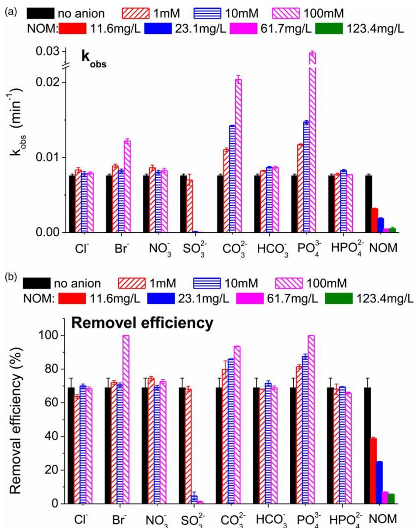
**Figure 2** | First-order degradation rate constant of phenol ( $k_{obs}$ ) and phenol removal efficiency after 140 min of reaction in the presence of different matrix species.
