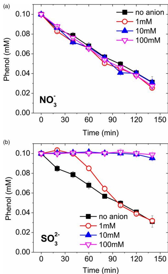
**Figure 3** | Impacts of  $\text{NO}_3^-$  and  $\text{SO}_3^{2-}$  on phenol oxidation by TAP. Experimental conditions:  $[\text{PS}]_0 = 10 \text{ mM}$ ,  $[\text{Phenol}] = 0.1 \text{ mM}$ , and  $T = 50^\circ \text{C}$ .
