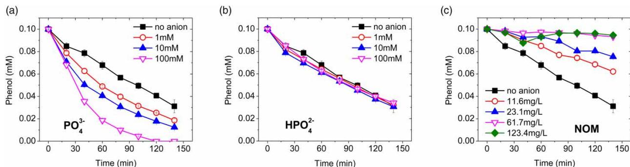
**Figure 5** | Impacts of PO<sub>4</sub><sup>3-</sup> (a), HPO<sub>4</sub><sup>2-</sup> (b) and NOM (c) on phenol oxidation by TAP. Experimental conditions: [PS]<sub>0</sub> = 10 mM, [Phenol] = 0.1 mM, and T = 50 °C.
