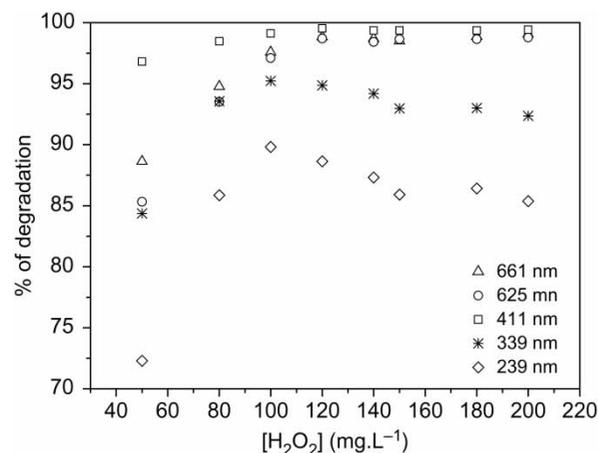
Figure 3 | Optimization of [H<sub>2</sub>O<sub>2</sub>]. Conditions: [Fe] of 1 mg·L $^{-1}$ , pH 3–4 and time of 1 h.
