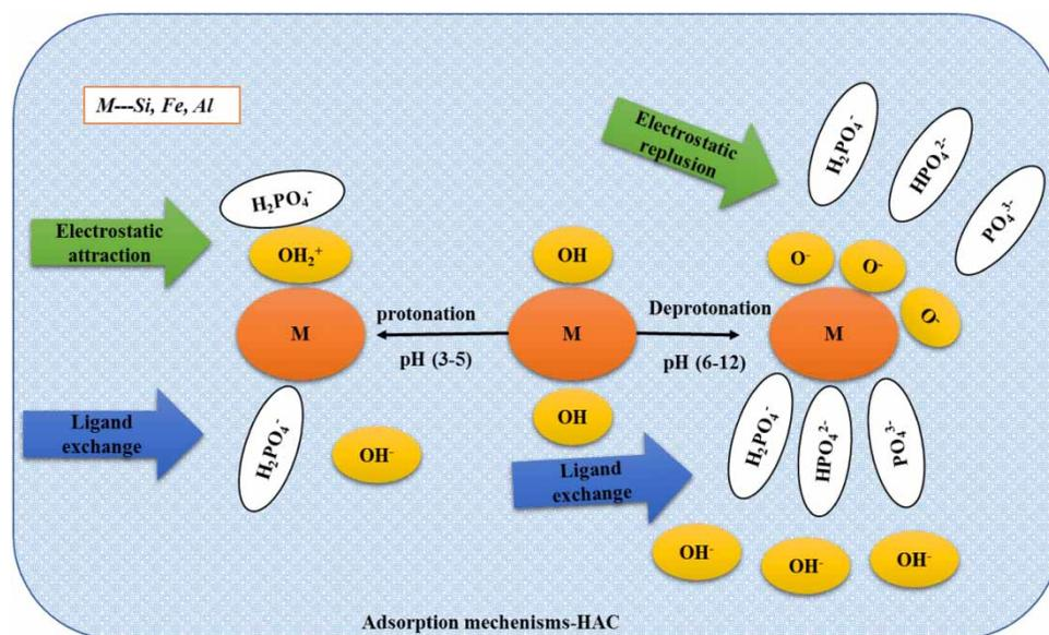
**Figure 5** | Proposed mechanisms for the removal of phosphate onto HAC at different initial solution pHs.
