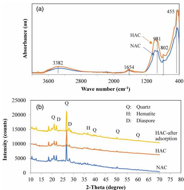
**Figure 2** | FTIR (a) and XRD (b) spectra of the NAC and HAC.
