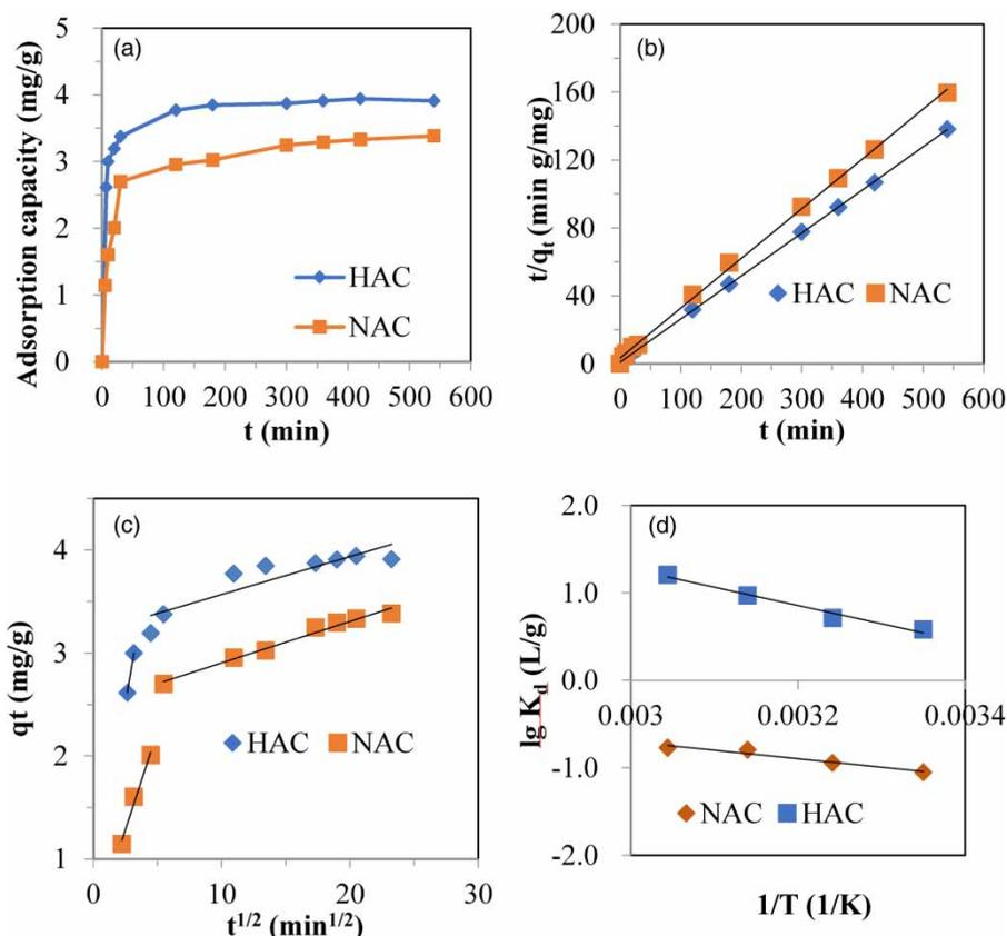
**Figure 3** | Effect of contact time on phosphate removal by HAC and NAC (a), pseudo-second-order model (b), intra-particle diffusion equation (c), and thermodynamics (d) (contact time = 0–540 min, initial concentration = 20 mg/L,  $T = 25\text{--}55\text{ }^{\circ}\text{C}$ ).
