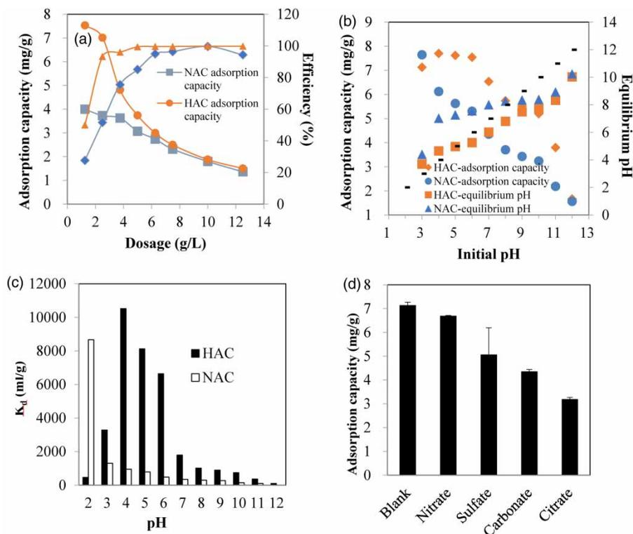
**Figure 4** | Effects of dosage (a) and initial pH (b) on phosphate adsorption onto the NAC and HAC. Distribution coefficient of phosphate adsorption onto the NAC and HAC at different initial pH (c), and effect of coexisting anions on the phosphate adsorption by HAC (d). (Initial concentration = 20 mg/L, dosage = 1.25–12.5 g/L, pH = 2.00–12.00, concentration of coexisting anions = 0.01 M).
