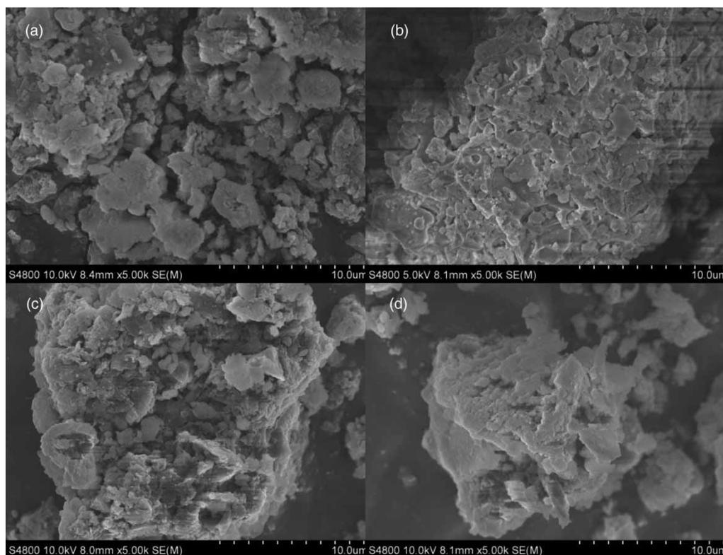
**Figure 1** | SEM images (acceleration voltage: 5.0 kV and 5,000 magnification) of the NAC (a) and after phosphate adsorption (c), HAC (b) and after phosphate adsorption (d).
