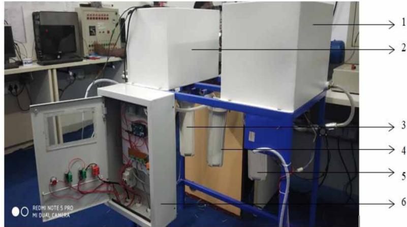
Figure 5 | Real time experimental setup of single stage pilot scale RO system.
