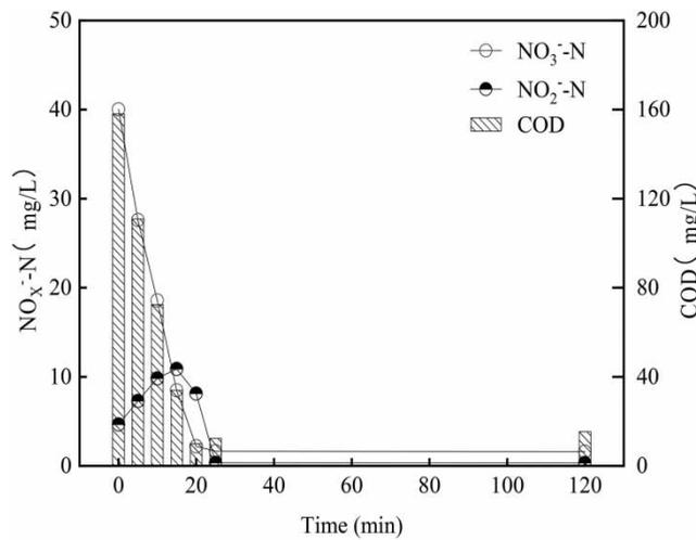
Figure 2 | Nitrogen conversion on 11th day via in-situ tests.
