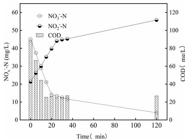
**Figure 3** | Nitrogen conversion on 90th day via in-situ tests.
