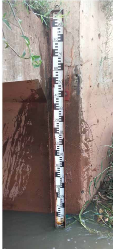
Figure 3 | Water level staff gauge located in the primary Lubigi channel at the Hoima Road box culvert crossing.
