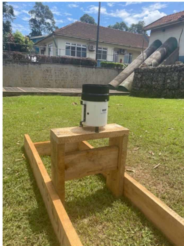
Figure 2 | Installed tipping bucket rain gauge mounted 50 cm above ground.
