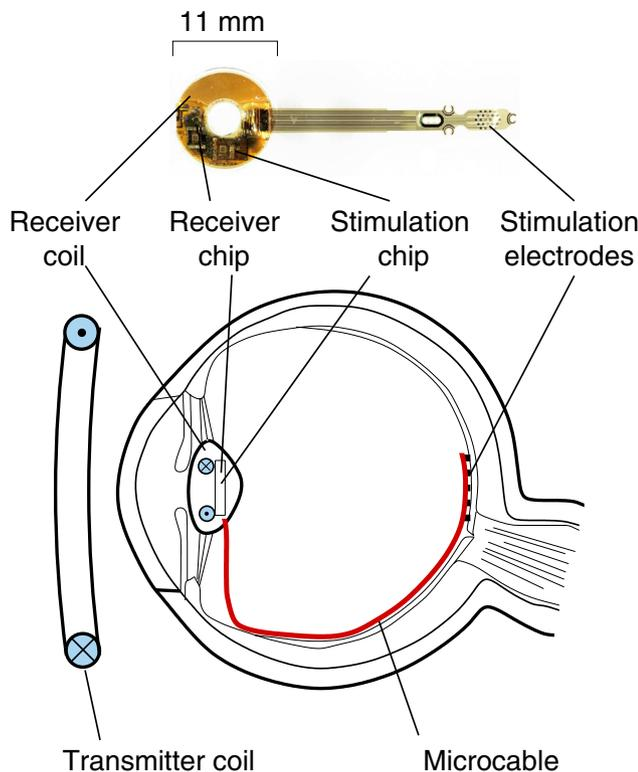
**FIGURE 1.** Schematic representation of an eye with a retinal implant. A receiver coil within the eye picks up the electromagnetic signals sent by the transmitter coil outside the eye and passes them to a receiver microchip. A custom-made stimulator chip generates the stimulation pulses and activates the selected electrodes placed on the epiretinal surface.
