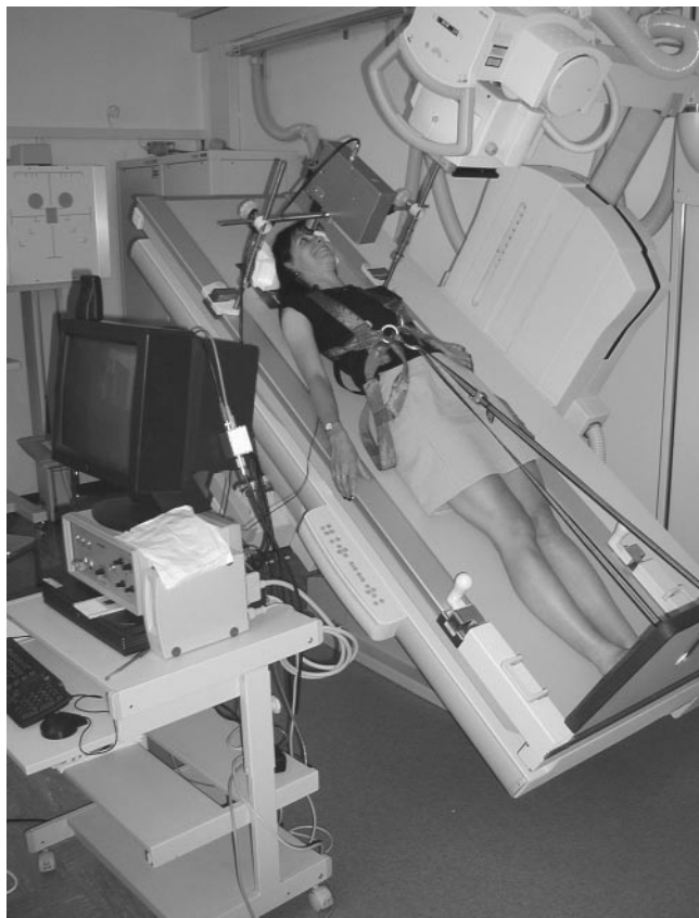
FIGURE 1. The LDF placed in front of the tested subject's eye is mechanically connected to the table. The computer-based data-acquisition system is at the bottom left in the photograph.
