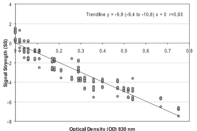
FIGURE 7. Data points of all filters of both subjects after correction for their offset are plotted and a trend line is fitted into the data points.  $P < 0.001$ .
