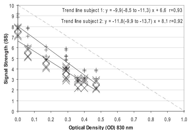
FIGURE 4. SS plotted against effective  $OD_{\lambda=830}$  values (single pass) of scattering filters. Large symbols: subject 1; small symbols: subject 2. Both the trend lines (black solid) and a straight line with a slope of  $-10$  (gray dashed) are included in the sets of data points.  $P < 0.001$ .
