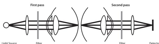
FIGURE 1. Schematic illustration of the first and second passes in OCT scanning with a filter placed in front of the eye.
