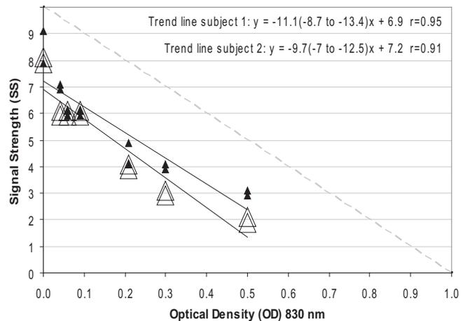
FIGURE 6. SS plotted against effective  $OD_{\lambda=830}$  values (corresponding to single pass) of defocusing lenses. *Open symbols*: subject 1; *filled symbols*: subject 2. Both the trend lines (*black solid*) and a straight line with a slope of  $-10$  (*gray dashed*) are included in the sets of data points.  $P < 0.001$ .
