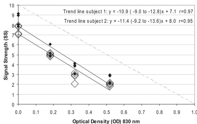
FIGURE 2. SS plotted against effective  $OD_{\lambda=830}$  values (single pass) of absorptive filters. Open symbols: subject 1; filled symbols: subject 2. Both trend lines (black solid) and a straight line with a slope of  $-10$  (gray dashed) are included in the sets of data points. The Pearson's correlation coefficients ( $r$ ) of the data, as shown in the figure, are statistically significant ( $P < 0.001$ ).
