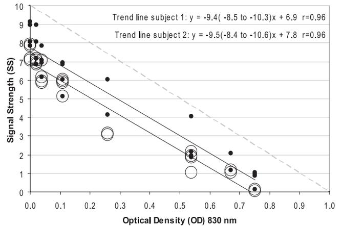
FIGURE 3. SS plotted against effective  $OD_{\lambda=830}$  values (single pass) of reflective filters. Open symbols: subject 1; filled symbols: subject 2. Both trend lines (black solid) and a straight line with a slope of  $-10$  (gray dashed) are included in the sets of data points.  $P < 0.001$ .
