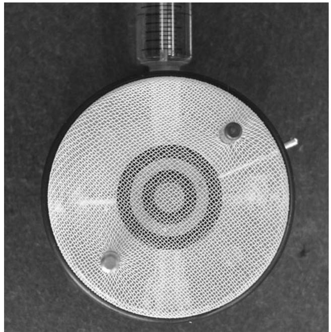
**FIGURE 1.** The nylon-covered hemichamber surface on which the complete annulus of rabbit I-CB was positioned. The concentric O-rings define a circular trough of 0.5 mL that bathes one side of the tissue. The inner O-ring sits within a notch on a central post of 4-mm diameter that occludes the pupil. After the I-CB was centered on the O-rings, a complementary hemichamber with matching O-rings (Fig. 2) was lowered on the alignment pins shown in the photograph.
