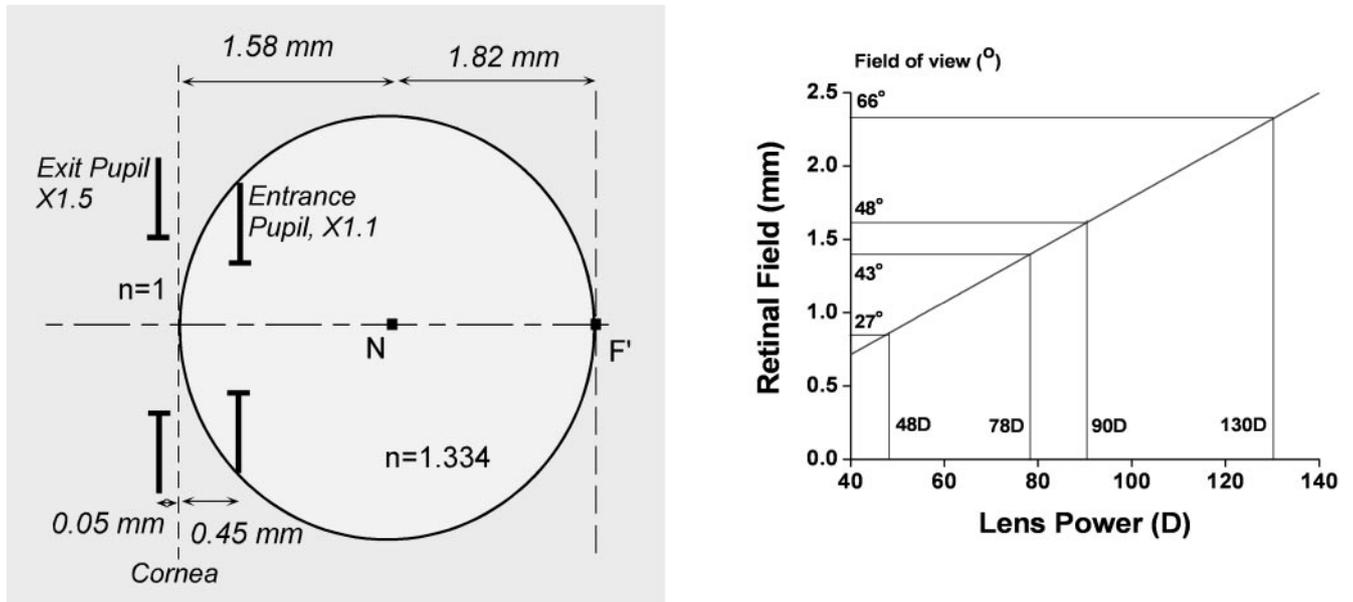
FIGURE 2. *Left:* reduced paraxial model of the mouse eye. The model was used to calculate the field of view as a function of auxiliary lens power, and it was derived from the complete paraxial model of Remtulla and Hartlett.<sup>39</sup> *Right:* The model predicts that 90-D auxiliary lens provides a field of view of approximately 48°.
