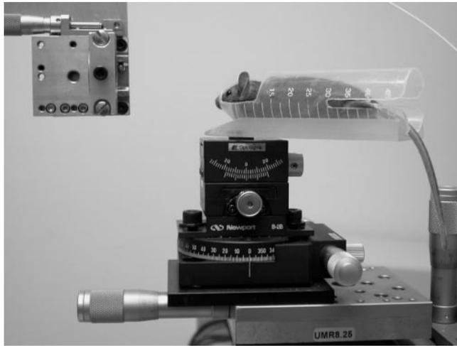
**FIGURE 4.** The mouse was held in a cylindrical holder made from 30-mL syringes. The position of the mouse was adjusted to align the optical axis of the mouse eye with the axis of the delivery system by using 6- $\mu$ m screws.
