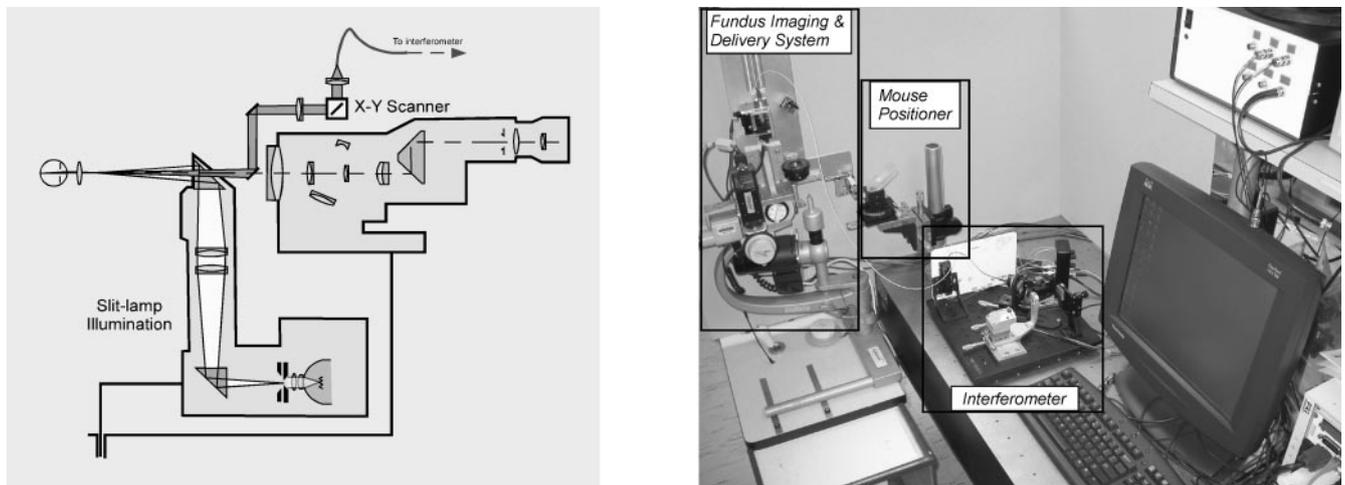
**FIGURE 1.** *Left:* general optical design of the imaging system; *right:* the mouse fundus and OCT imaging system, including fundus imaging with a digital camera attached to the photographic port of the slit lamp, the OCT beam delivery system, the six-axis mouse positioner, and the interferometer.
