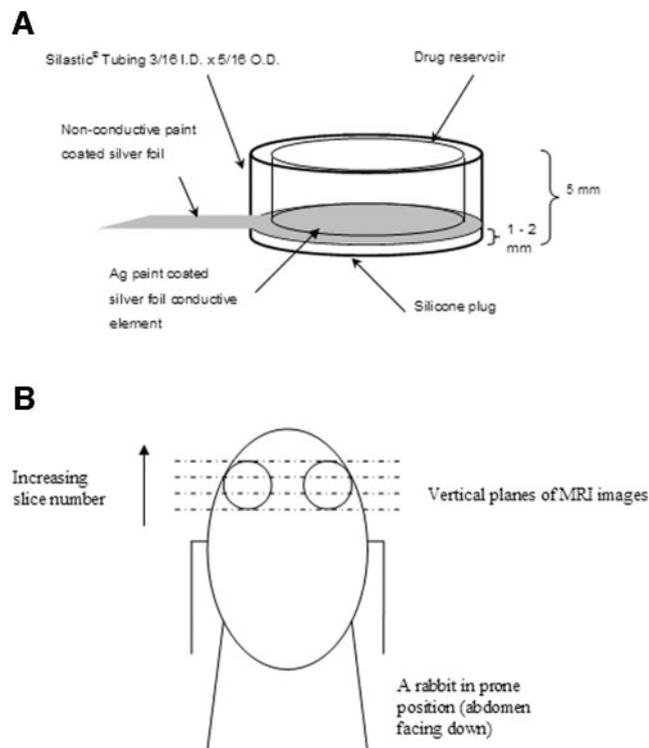
FIGURE 1. (A) Donor electrode device configuration. (B) MR imaging planes and orientation (diagram not to scale).
