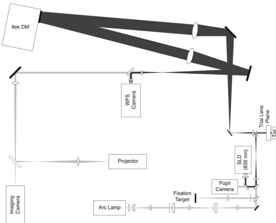
FIGURE 1. Flood-illuminated adaptive optics fundus camera at UC Davis. *Dark gray*: AO control loop; *light gray*: imaging and vision testing paths.
