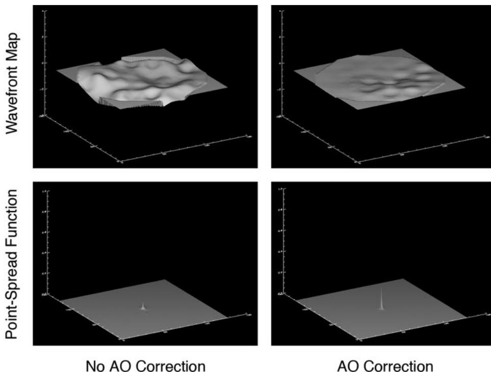
**FIGURE 2.** Wavefront (WF) and point-spread function (PSF) plots before and after AO correction over a 7-mm pupil. The WF became flatter after AO correction due to a decrease in RMS error by a factor of 3. The Strehl ratio of the PSF increased by a factor of 3.
