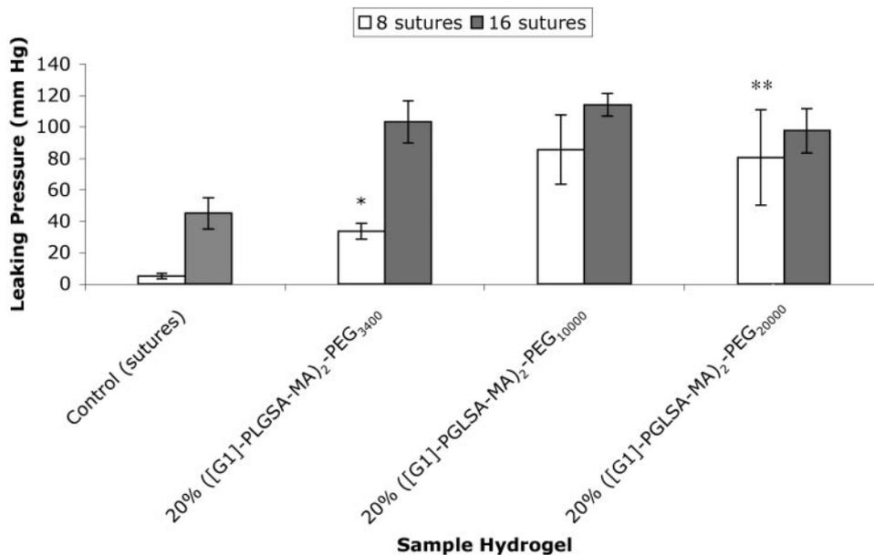
**FIGURE 3.** Leaking pressures for PKP autografts sealed with either 8 or 16 10-0 nylon sutures and the three different biodegradable adhesive formulations at 20% wt/vol. All the adhesives were evaluated in enucleated porcine eyes ( $n = 3$  per formulation). All samples are significant ( $P < 0.02$ ) compared with the 16-suture control group, unless otherwise noted.  $*P = 0.11$  and  $**P = 0.08$  when compared with the 16-suture control group.
