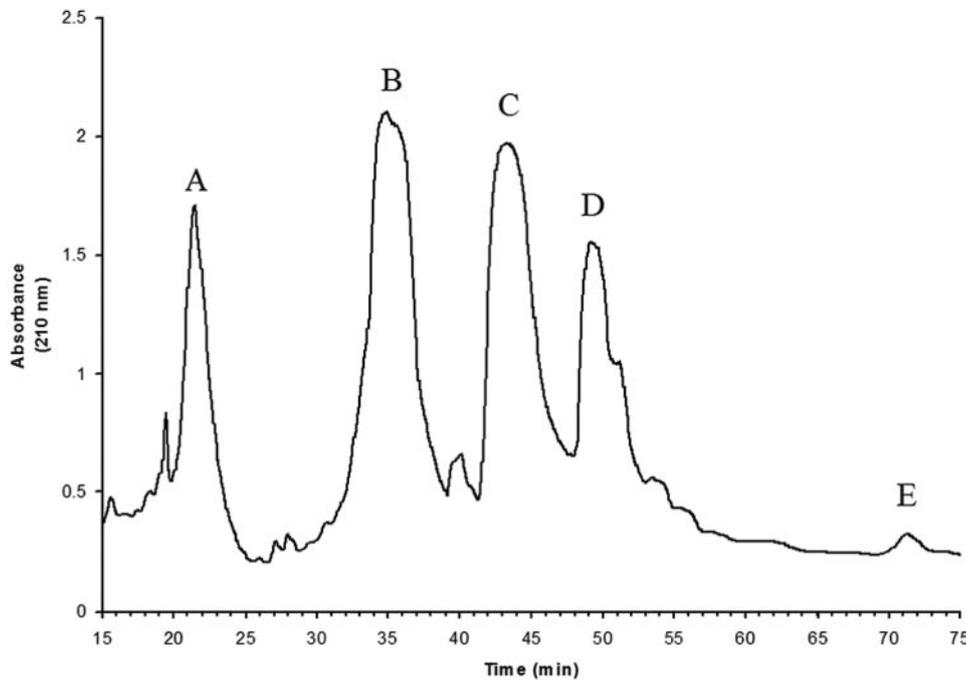
**FIGURE 5.** An HPLC chromatogram for separation and purification of these two proteins from the tears of eyes with pterygium. A 10.8-kDa protein was found in peak D at a retention time of 49.2 minutes, and a 12.7-kDa protein was observed in peak E at a retention time of 71.6 minutes.
