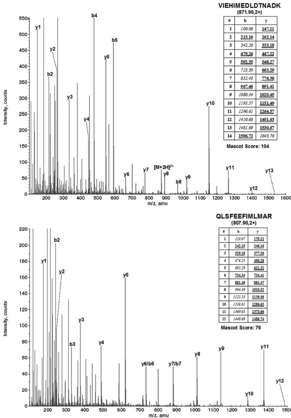
FIGURE 7. MS/MS spectra showed the fragment ions from one doubly charged precursor ion at  $m/z$  871.90 (VIEHIMEDLDTNADK) and another doubly charged precursor ion at  $m/z$  807.90 (QLSFEEFIMLMAR), both originating from S100 calcium-binding protein A9. Peaks corresponding to  $y$  and  $b$  ions are marked.
