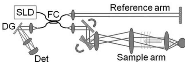
FIGURE 1. The FD OCT interferometric setup used to image the mouse retina.
