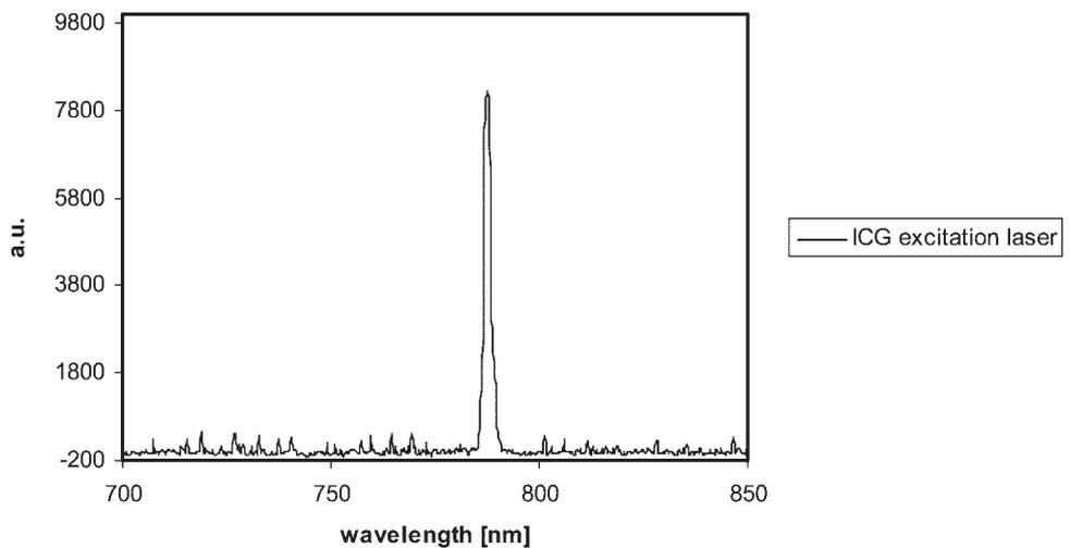
**FIGURE 9.** Spectrometer analysis of NIR fluorescence diode laser emission. The laser power was reduced by a series of gray filters (transmission  $1.4 \times 10^{-4}$ ). The laser peak is detected at 787 nm without sideband emissions. xAxis: wavelength in nanometer; y-axis: laser power in arbitrary units.
