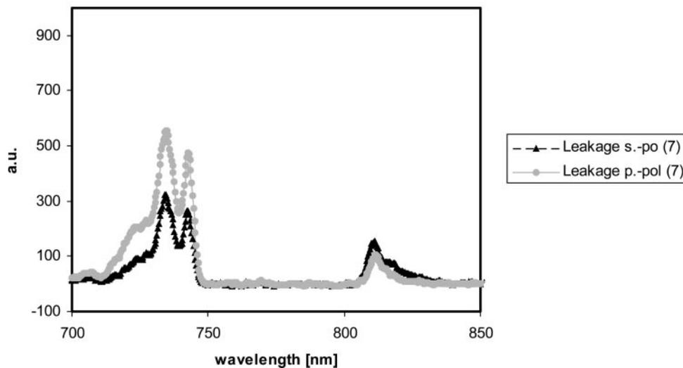
FIGURE 10. Leakage of the HRA imaging system combining barrier filter leakage and output coupler reflectance. Although the laser peak is completely suppressed, there is some sideband emission in the range of  $6.2 \times 10^{-6}$  (p-polarized) and  $6.7 \times 10^{-6}$  for s-polarized laser light measured at the standard laser power (switch position 7). *x*-Axis: wavelength in nanometers, *y*-axis: leakage in arbitrary units.
