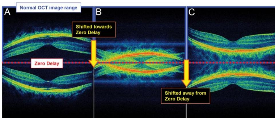
appears brightest when it is near 0 delay (Fig. 1C) and weakest when it is farther from it (Fig. 1A). Most commercial instruments are designed to work with the retina placed posterior to the 0-delay line (Fig. 1A), to enhance sensitivity for imaging epiretinal membranes or vitreal detachments. Finally, instruments have a maximum axial scan depth range over which imaging can be performed.
