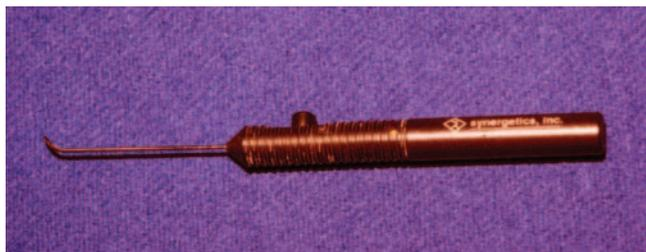
FIGURE 1. Custom-made device used to insert implants through a retinotomy into the subretinal space. Inserter made by Michael Ault (Synergetics, Inc., O'Fallon, MO).
