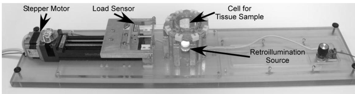
**FIGURE 2.** Optomechanical lens stretching system. The stepper motor, load sensor, tissue holder, and retroillumination source are labeled. The tissue is placed inside the cell and then mounted on eight individual hooks.
