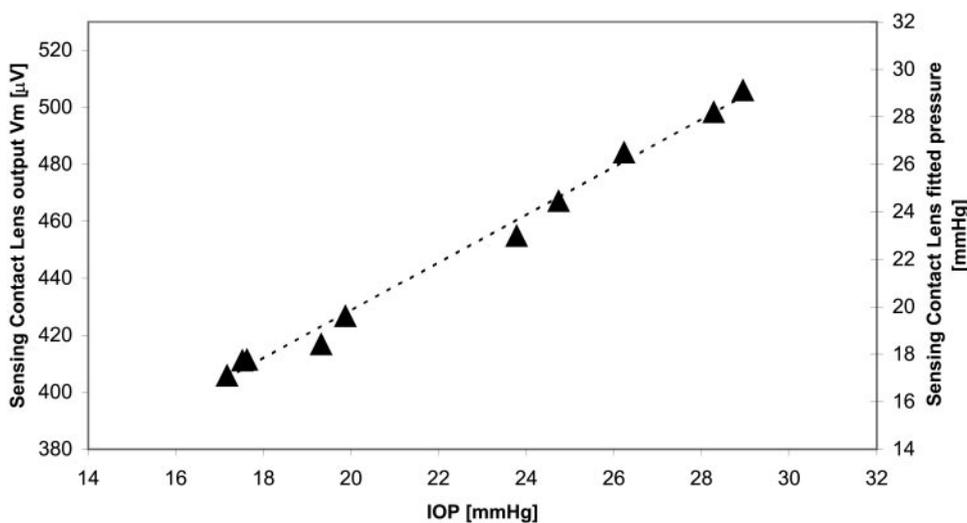
FIGURE 5. Static calibration graph. The output signal  $V_m$  of the sensing contact lens has an experimental fitted sensitivity of  $8.37 \mu V/mm Hg$ , and it can be seen that it showed good linear fit. For linear regression,  $R^2 = 0.992$ .
