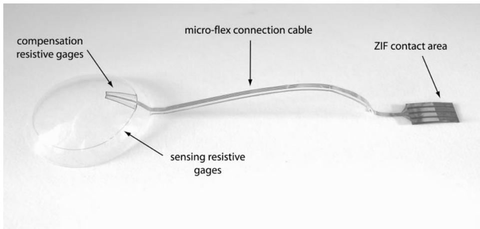
**FIGURE 1.** The sensing contact lens. Shown is the location of the active gauges, which are placed circumferentially for sensing changes in the corneal curvature due to IOP, and the passive gauges for thermal compensation, which are placed radially, where no strain should be measured. The gauges are made of thin metallic film patterned by surface micromachining on a polyimide microflex substrate, which is then embedded into the silicone soft contact lens.
