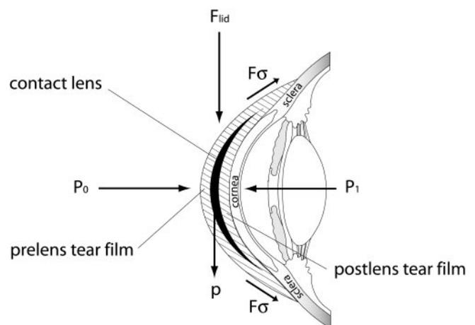
**FIGURE 2.** The five major physical forces acting on a contact lens:  $P_0$ , atmospheric pressure;  $P_1$ , hydrostatic pressure of the postlens tear film;  $F_\sigma$ , surface tension of the prelens tear film;  $p$ , lens weight; and  $F_{\text{lid}}$ , lid force.
