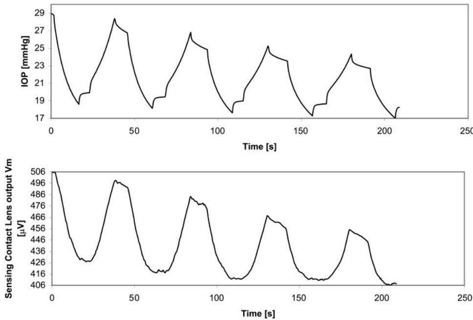
FIGURE 4. Record of the IOP and the sensing contact lens output signal  $V_m$  during liquid injection-ejection cycles. The sensing contact lens followed the pressure sensor well and showed the potential for continuously monitoring IOP in enucleated porcine eyes.
