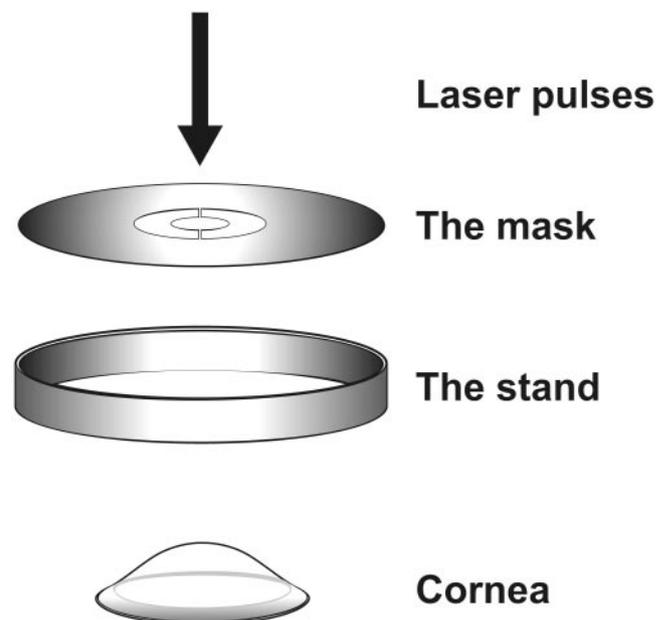
FIGURE 1. Donut- or ring-shaped laser ablation masking system set up. A human cornea is placed beneath a circular stand used to hold the mask. The area without the metal masking (i.e., donut shape) is ablated with an excimer laser.
