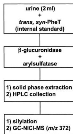
Fig. 3. Analytical scheme for quantitation of *r*-1,*t*-2,3,*c*-4-tetrahydroxy-1,2,3,4-tetrahydrophenanthrene (*trans*, *anti*-PheT) in human urine. *trans*, *syn*-PheT, *r*-1,*t*-2,4,*c*-3-tetrahydroxy-1,2,3,4-tetrahydrophenanthrene; HPLC, high-performance liquid chromatography; GC-NICI-MS, gas chromatography-negative ion chemical ionization-mass spectrometry.
